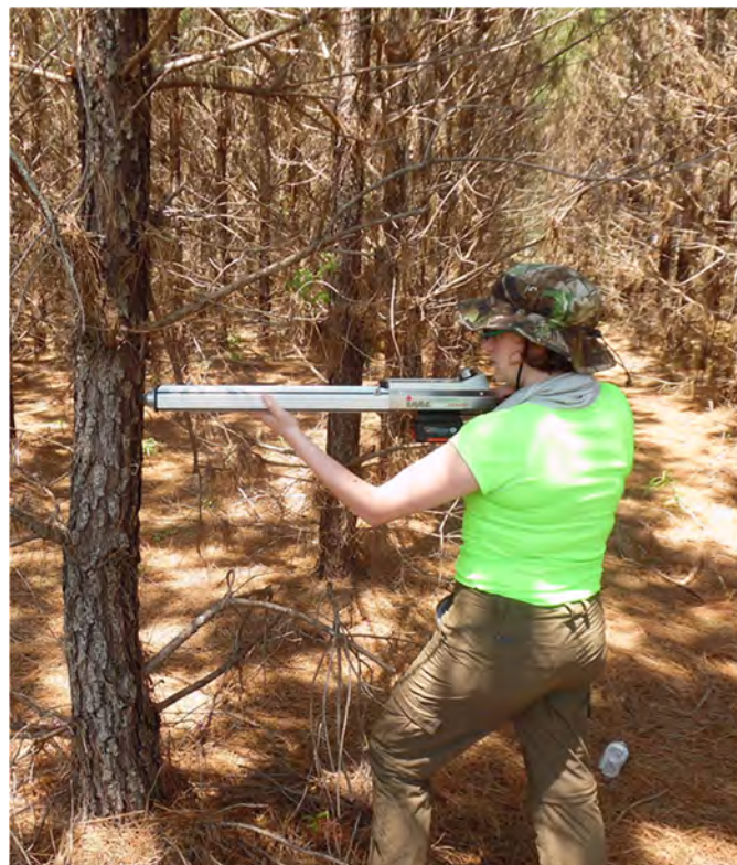
Picture 1. The Resistograph tool is a surrogate for wood density assessment and measures the resistance (in amplitude) to drill a fine needle at a constant speed through wood. With an expert operator like April Meeks, about 80 trees can be assessed in an hour.
