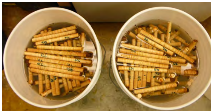
Pictured above: 12 mm cores from study trees saturating in buckets for specific gravity measurements.
