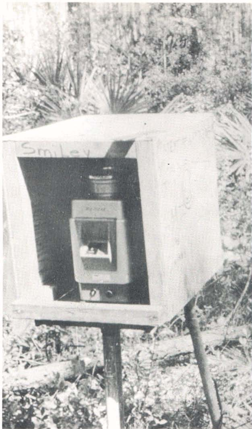
Large, intensive wood studies are under way by a number of industries. Pictured is a high sensitivity electric balance specially adapted to field studies by Continental Can Company. Also shown are the disks from one of their several hundred intensively sampled trees, used to determine the relationship between breast height and total tree values.
