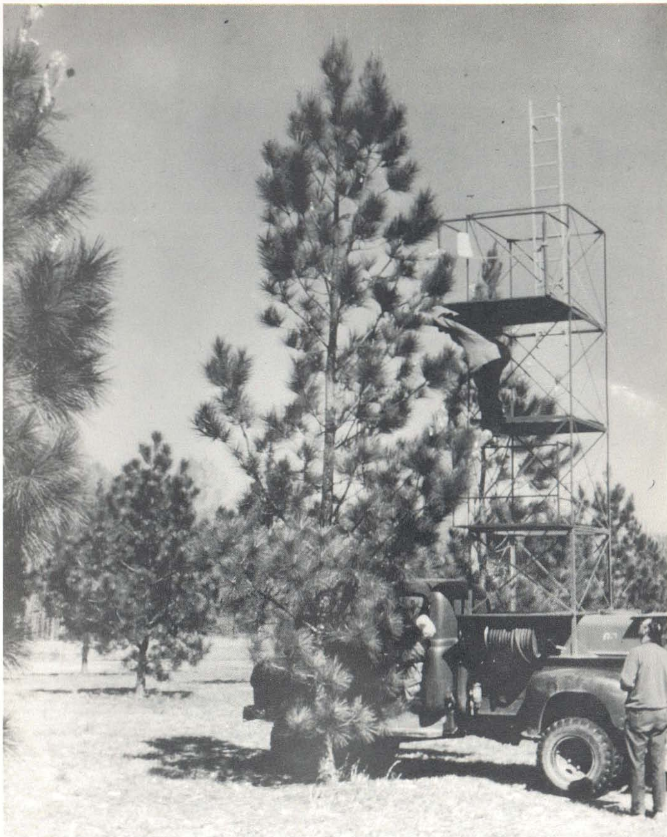
A major problem faced by the cooperating industries is to develop equipment for use in the seed orchards. Some unique equipment has been designed, especially to enable the control-pollinations necessary for progeny testing. There are nearly as many kinds of equipment as there are organizations; one "home developed" rig is shown at the International Paper Company orchard in South Carolina. Several industries have completed the pollinations necessary for progeny testing the seed orchards.
