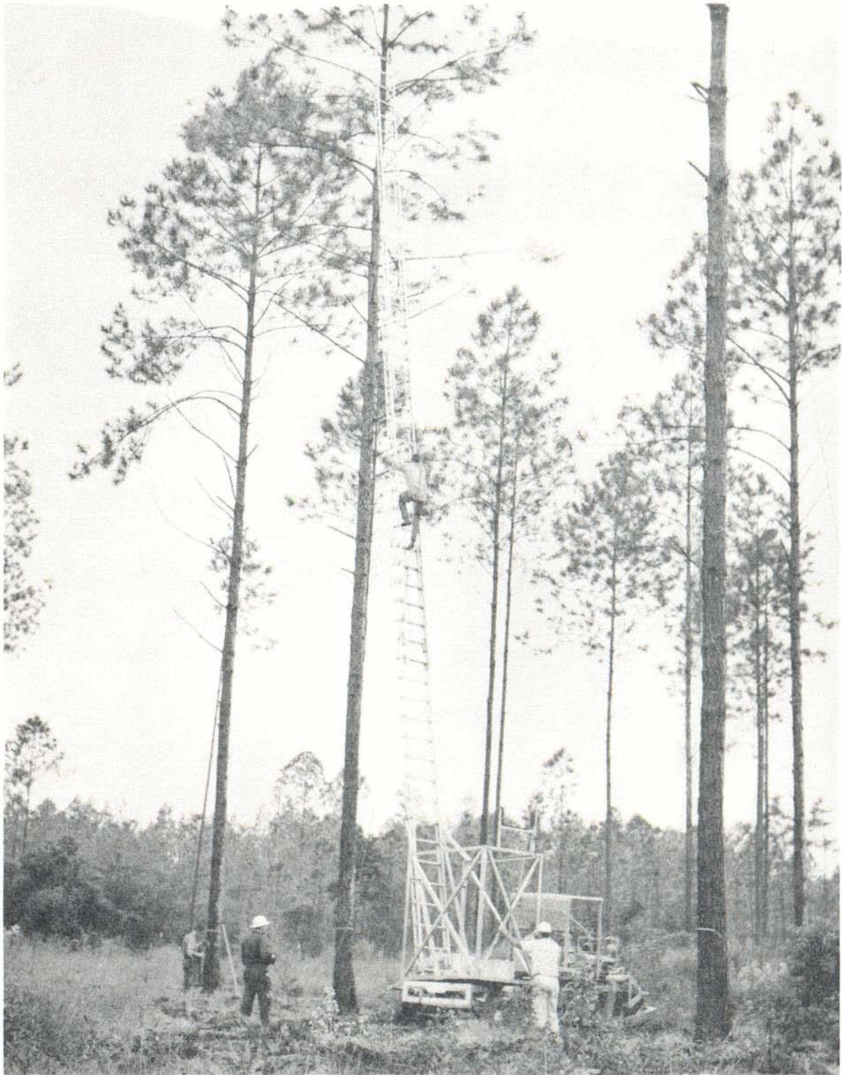
Fig. 12. A trailer-mounted ladder to climb large trees, such as those in a seed production area, was developed at Southland Experiment Forest of the International Paper Company. This ladder was used to make the bulk of the crosses necessary in the large pine heritability project.
