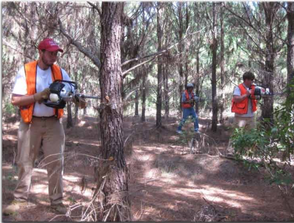
Cores from 1668 trees in the Plum Creek / CellFor clonal trials were collected and analyzed for wood properties associated with ethanol production.
