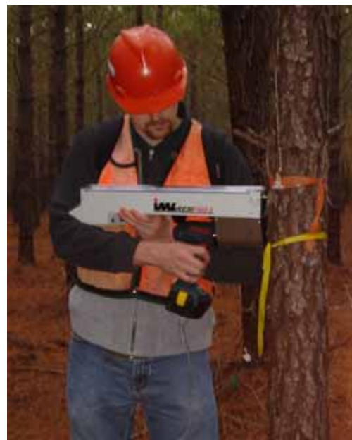
Figure 2. Tyler Eckard, a graduate student, measuring relative wood density of trees using the Resistograph in a clonal trial
