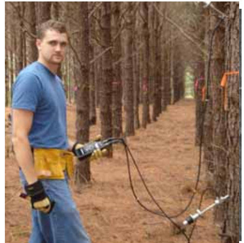
Figure 1. Measuring acoustic velocity for trees from a diallel test series with the TreeSonic
