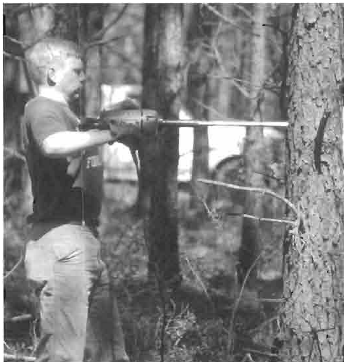
Robert Sykes uses an industrial drill to extract wood core samples from a field test in South Carolina
