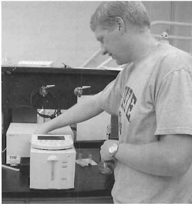
Back at the lab, Robert Sykes uses a UV-visible spectrophotometer to measure the absorbance of a solution of dissolved wood and acid, in order to determine lignin content.
