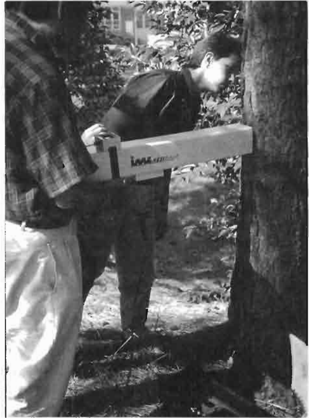
Paula Zanker assists as Dr. Fikret Isik uses the Resistograph to produce a density profile for a mature loblolly pine.
