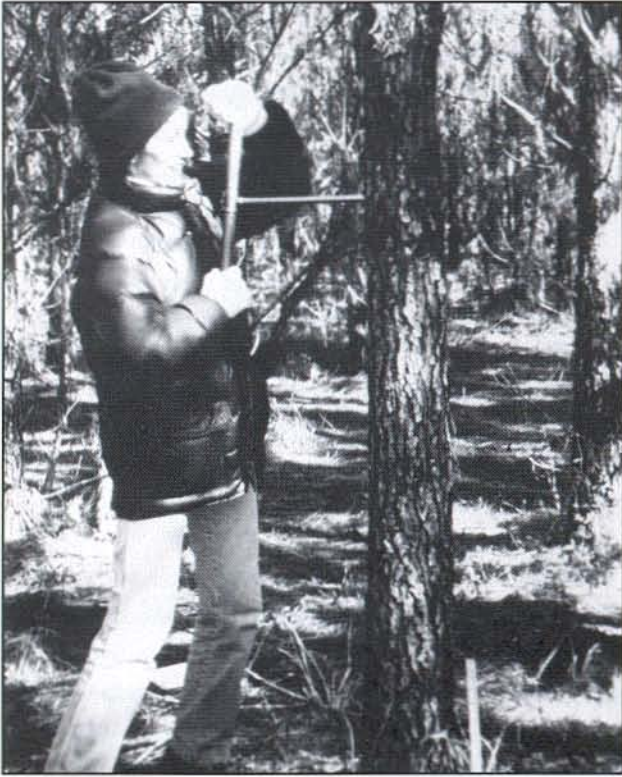
Barbara McCutchan extracts a 12mm increment core from a new third-cycle selection graded in one of Westvaco's progeny tests.
