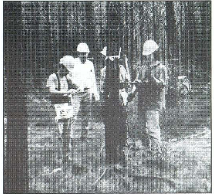
Wood sampling in Union Camp's Florida Loblolly Provenance/Progeny Trial to determine provenance and family variation in wood properties.
