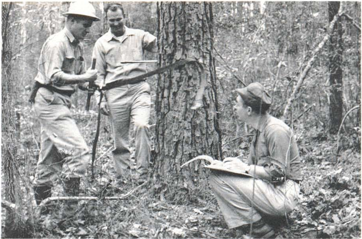
Figure 10. Taking the oversize cores is a "man-sized" job. A special starter is helpful in getting the bit into the tree. Paul Otterbach is shown in the act of releasing the starter.
