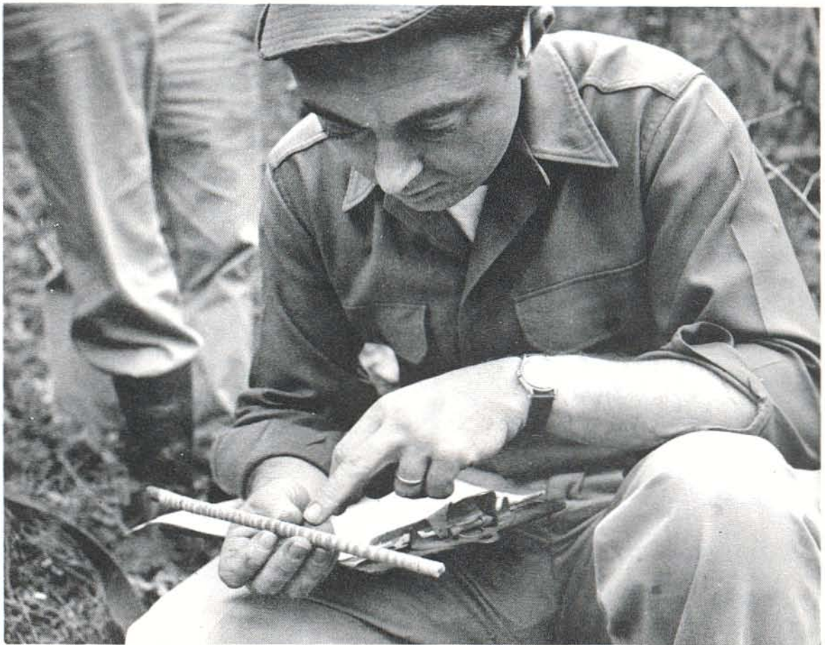
Figure 11. Bob McElwee here holds the oversize increment core used for samples of wood specific gravity and cellulose yield.
