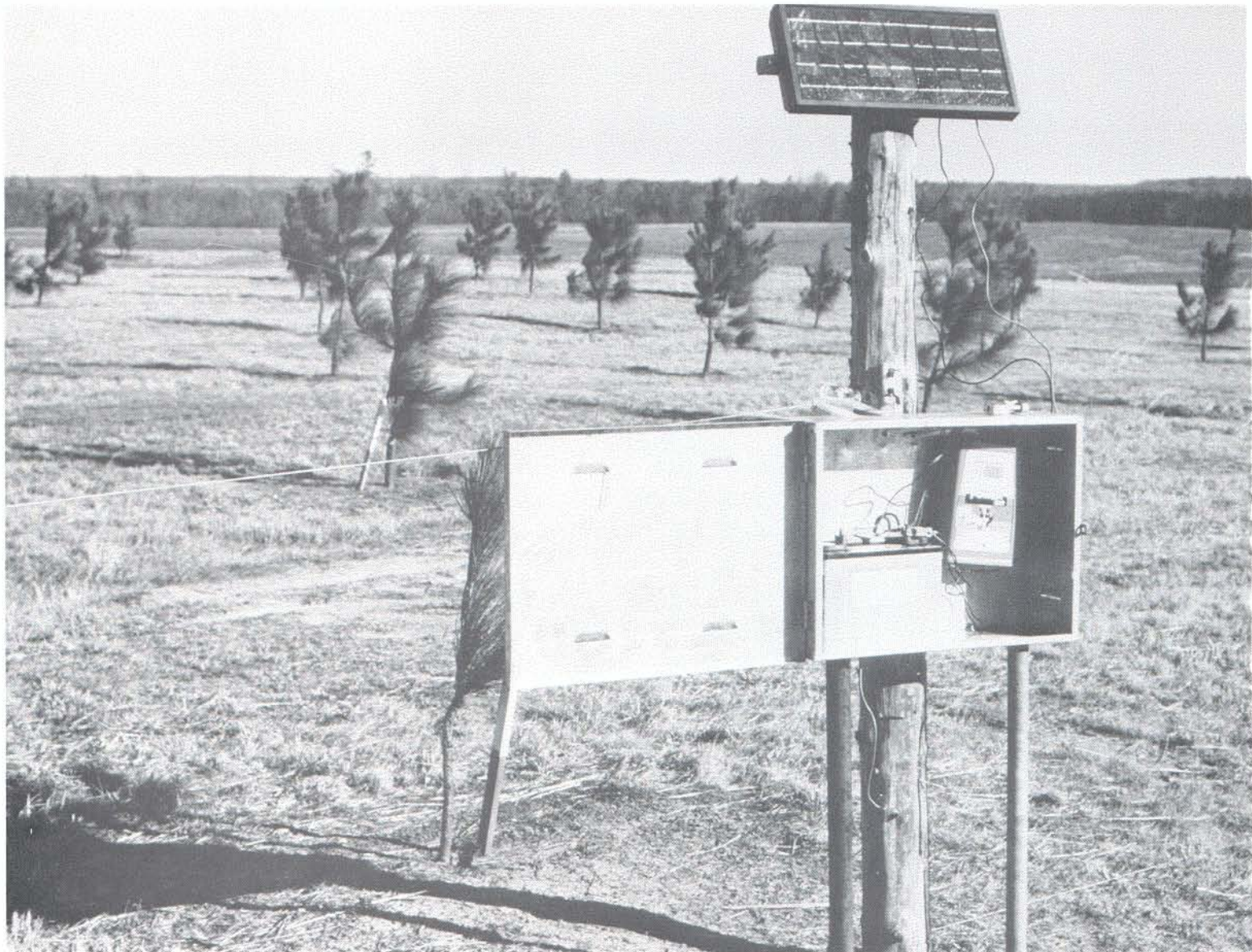
A solar powered electric fence is being used by Champion International to "discourage" deer from damaging a young seed orchard near Newberry, South Carolina.
