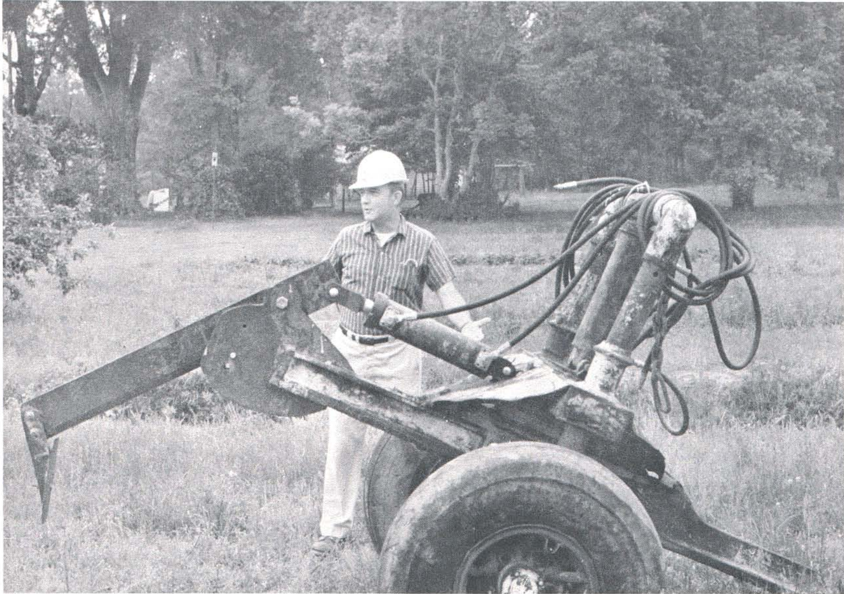
A converted fire plow makes an excellent subsoiler for International Paper Company. The coulter which cuts heavy roots is hidden by the tires. Beneficial effects of subsoiling include root pruning, and reduced soil compaction.
