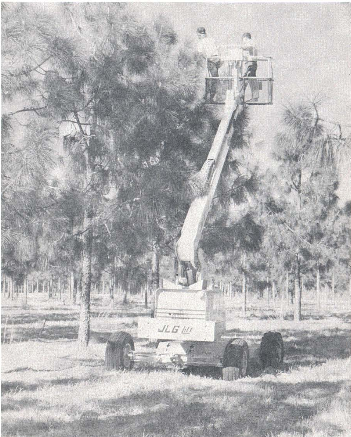
Lift vehicles are essential equipment in older orchards. Shown is a JLG lift in use at the North Carolina Forest Service longleaf orchard. Lift vehicles are used in cone harvest, control-pollination work, production inventories, and research activities.
