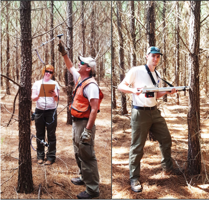
Image 1. Georgia Forestry Commission Staff completing wood quality measurements on 3 rd -Cycle pollen mix tests using TreeSonic (left) and Resistograph (right) to assess the wood stiffness and density, respectively, of parents in the CPMX5 series.
