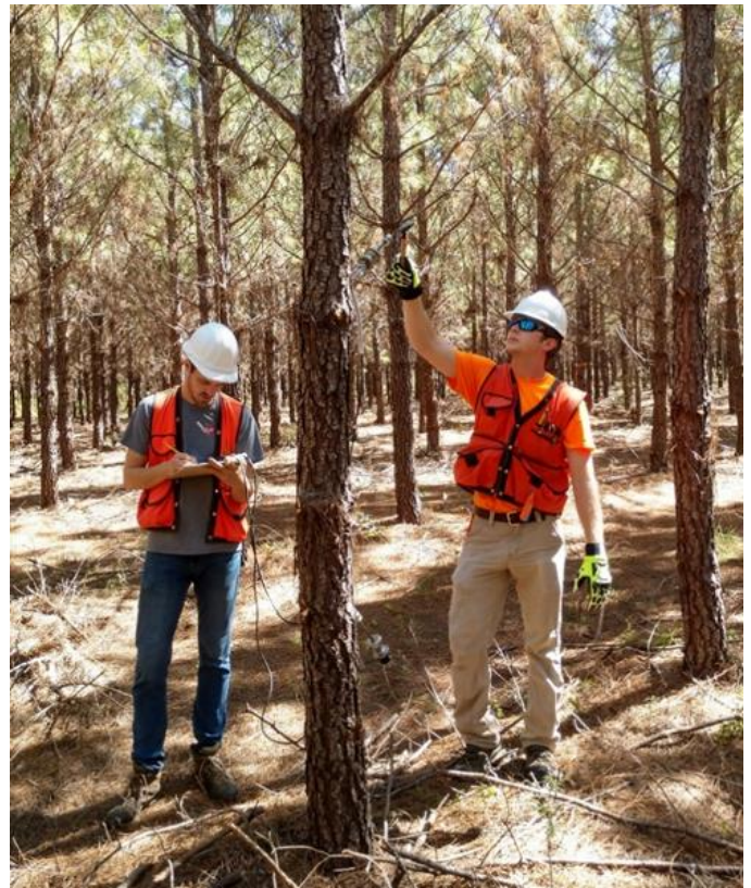
Image 1. The TreeSonic tool contains a probe that is tapped with a hammer and measures the time for the sound wave to pass through the stem. Faster acoustic wave values indicate stiffer wood. Peter McNeary (left) and Ben Maness (right), both undergraduate students pictured here measuring wood properties with the TreeSonic tool (photographed by Austin Heine).
