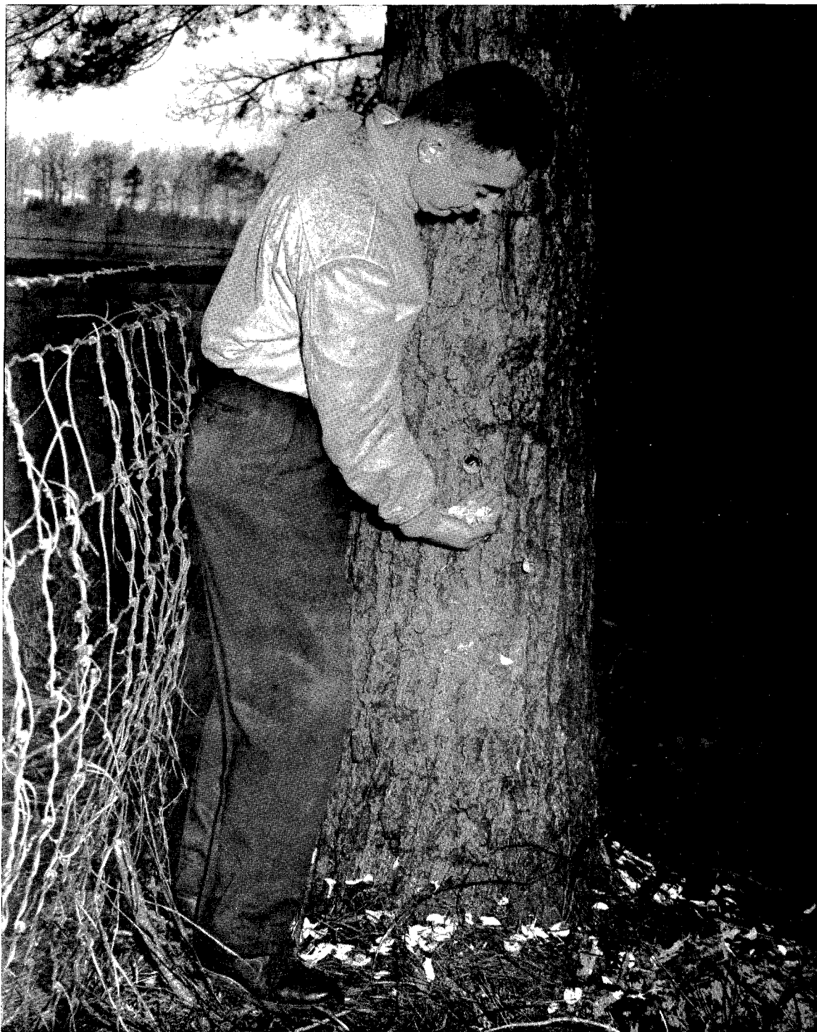
Special tools are needed to obtain specimens from living trees. Bob McElwee shows the kind of chips obtained with the Little Beaver attachment that will be used on tests of variation in pulp yields. (Photo - courtesy D. Davis, Champion Paper Co.)
