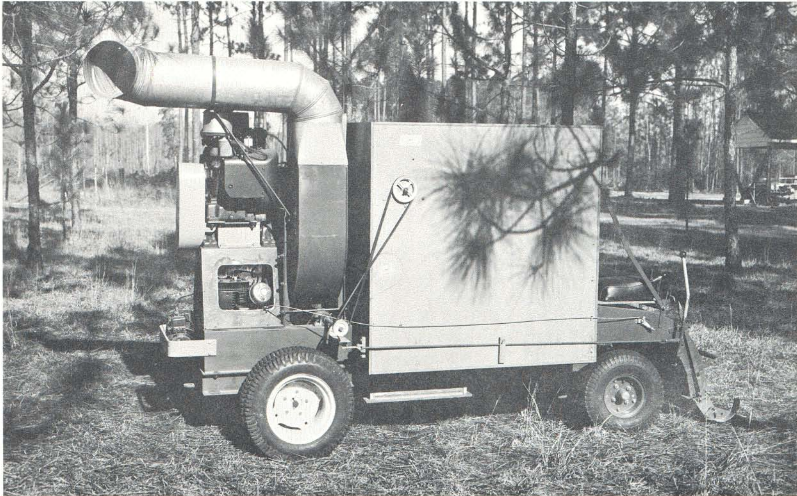
Figure 6. Some seed orchards have come into heavy production and it is essential to find a quick and efficient method of harvesting cones and seed. A "Seed Harvest Committee" from the Cooperative has been hard at work on this for two years. A prototype "vacuum principle" machine has been developed to pick up seeds from the ground and an operational model is now under construction. (Photo, courtesy of Barry Malac, Union Camp Corporation)
