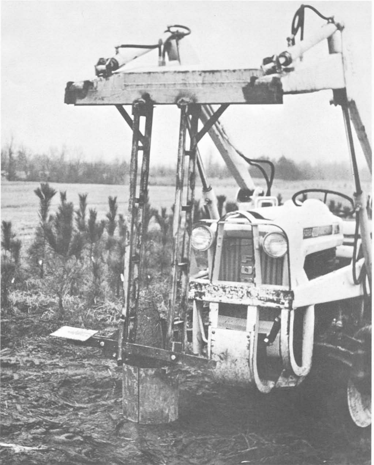
Many ingenious methods have been developed by members of the Cooperative to speed up their operations and to make them more efficient. This mechanized transplanter, developed at Tennessee River Pulp and Paper Company, has made transplanting of grafts faster and more economical. Similar systems have been developed at many of the Cooperative's seed orchards.
